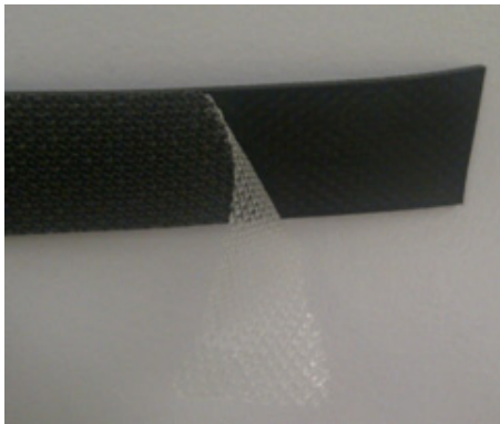
Figure 4-47: Exposing the tack side of the sealing tape
