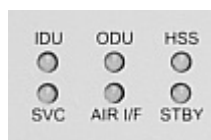
Figure 4-39: IDU-C Front Panel LEDs
